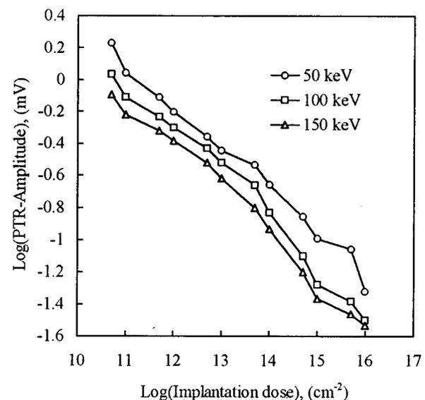
FIG. 3. Experimental dependencies of PTR amplitude on implantation dose for 50, 100, and 150 keV implantation energies taken at 10 kHz modulation frequency.
