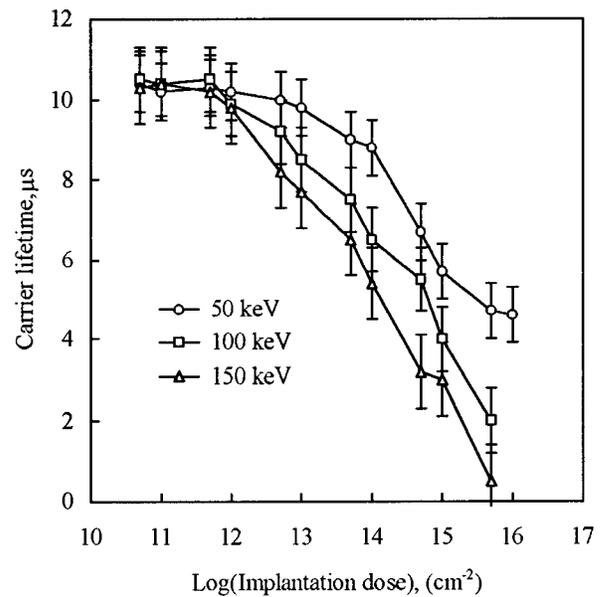
FIG. 2. Values of the minority carrier lifetime evaluated from the PTR amplitude and phase frequency responses as a function of implantation dose for implantation energies of 50, 100, and 150 keV.
