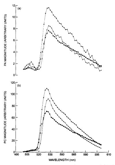
Fig. 4. Magnitudes of (a) PA and (b) PC spectral responses with a transverse electric field of 20 VDC: (--O--), quasi-random polarization; (-+--),  $E \perp C$ ; (--O--),  $E \parallel C$ . Light chopping frequency: 23 Hz; spectral resolution: 2 nm;  $T = 22^{\circ}$ C.
