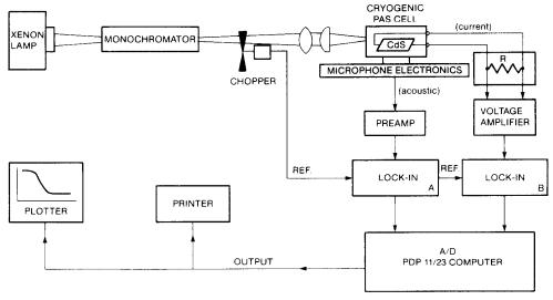
Fig. 1. Schematic diagram of the experimental apparatus for variable temperature PA and PC measurements.
