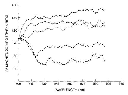
Fig. 3. Open-circuit PA magnitude of pure *n*-CdS single crystal with temperature as a parameter: ( $-\bigcirc$ -),  $T = 22^{\circ}$ C; ( $-\bigtriangleup$ -),  $T = -23^{\circ}$ C; (-+-),  $T = -73^{\circ}$ C; ( $-\times$ -),  $T = -116^{\circ}$ C; ( $-\diamondsuit$ -),  $T = -160^{\circ}$ C. Light chopping frequency: 23 Hz. Spectral resolution: 4 nm, randomly polarized.
