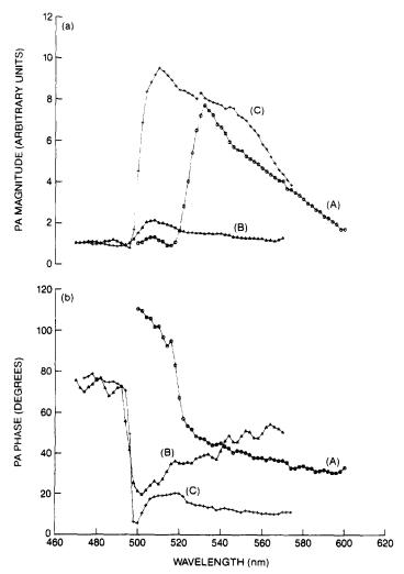
Fig. 6. Magnitudes (a) and phases (b) of PA with a transverse electric field of 20 VDC; curves (A):  $T = 22^{\circ}$ C; curves (B):  $T = -160^{\circ}$ C smoothened spectra; curves (c):  $T = -160^{\circ}$ C, after fracture. Light chopping frequency: 23 Hz; spectral resolution: 2 nm. All magnitude spectra normalized to the same value at 470 nm.
