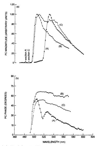
Fig. 7. Magnitudes (a) and phases (b) of PC spectra with a transverse electric field of 20 VDC; curves (A):  $T = 22^{\circ}$ C; curves (B):  $T = -160^{\circ}$ C; curves (C):  $T = -160^{\circ}$ C, after fracture. Light chopping frequency: 23 Hz; spectral resolution: 2 nm. All magnitude spectra normalized to the same peak value.
