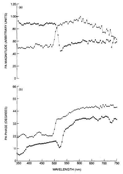
Fig. 2. Open-circuit PA spectra of pure *n*-CdS single crystal:  $(-\bigcirc -)$ ,  $T = 18^{\circ}$ C;  $(-\triangle -)$ ,  $T = -160^{\circ}$ C. Light chopping frequency: 30 Hz. Spectral resolution: 8 nm, randomly polarized: (a) magnitude; (b) phase.
