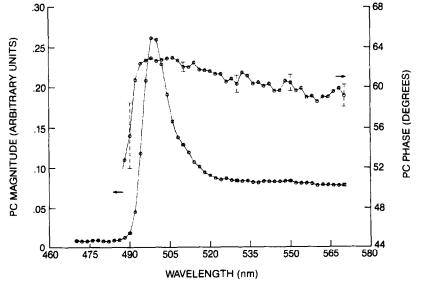
Fig. 10. PC signal magnitude and phase recorded at 2f with intact pure *n*-CdS in the presence of a transverse AC electric field of 20 V peak-to-peak;  $T = -160^{\circ}$ C.
