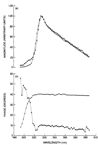
Fig. 9. Magnitudes (a) and phases (b) of PA and PC spectra at 2f with a transverse AC electric field of 20 V peak-to-peak and quasi-randomly polarized unmodulated light. Electric field modulation frequency f = 23 Hz; spectral resolution: 2 nm;  $T = 20^{\circ}$ C. (--O--), PA spectrum; (-- $\Delta$ --), PC spectrum. Magnitudes matched arbitrarily at 532 nm.
