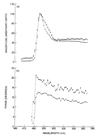
Fig. 11. Magnitudes (a) and phases (b) of PA and PC spectra at 1*f* with a transverse AC electric field of 20 V peak-to-peak and quasi-randomly polarized unmodulated light. Electric field modulation frequency f = 23 Hz; spectral resolution: 2 nm;  $T = -163^{\circ}$ C. (-O-), PA spectrum; (- $\Delta$ -), PC spectrum. Magnitudes matched arbitrarily at 498 nm.
