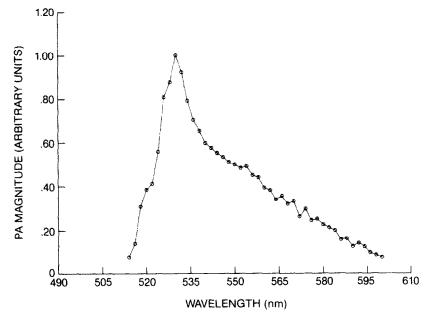
Fig. 8. PA magnitude with a transverse AC electric field of 20 V peak-to-peak and quasi-randomly polarized unmodulated light. Electric field modulation frequency: 23 Hz; spectral resolution: 4 nm:  $T = 20^{\circ}$ C.
